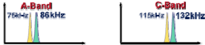
Figure 10 PL-20 Carrier Frequencies
